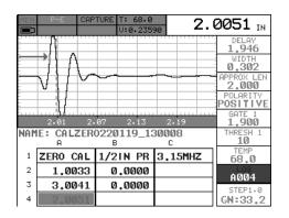
1) Press the **UP, DOWN, LEFT, & RIGHT** arrow keys multiple times using the left button wheel to scroll the cursor to an empty L-REF cell in column A, row #4 – 6.
