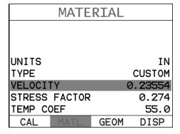
1) Press the **MENU** key multiple times to tab right and the **ESC** key multiple times to tab left until the **MATL** menu is highlighted and displaying the sub
