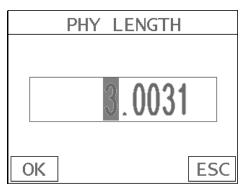
6) Press the UP, DOWN, LEFT, & RIGHT arrow keys multiple times using the left or right button wheel to scroll the highlighted value until the desired PHY LENGTH is correctly displayed.
