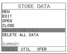
2) Use the **UP** and **DOWN** arrow keys on the left button wheel to scroll through the sub menu items until **DELETE ONE FILE** is highlighted.
