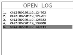
7) Press the **ENTER** key to display the Cal Zero group data files in the project.
