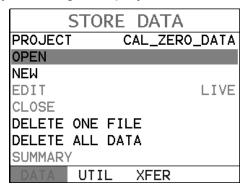
6) Press the **UP** and **DOWN** arrow keys multiple times using the left button wheel to scroll through the menu items until **OPEN** is highlighted.
