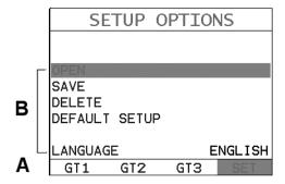
1) Press the **MENU** key once to activate the menu items tab. Press the **MENU** key multiple times to tab right, and the **ESC** key multiple times to tab left until the desired tab group is highlighted and displaying the submenu items. Alternatively, press the **LEFT** and **RIGHT** arrow keys multiple times using the left button wheel. The tab groups are illustrated above (A).
