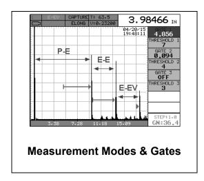
As stated above, the **MAX II** has a total of three gates depending on the measurement mode selected. The photo above illustrates the mode and number of gates needed for each measurement mode. One gate is used in pulse-echo, two gates for echo-echo, and 3 gates for echo-echo verify. The gates are fully independent, and starting positions and thresholds are the only adjustments available for each gate.
