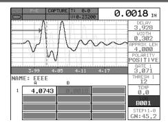
1) Press the MEAS key once to activate measure menu items. Press the MEAS key multiple times to move down and the ESC key multiple times to move up until the LOG cell is highlighted. Alternatively, press the LEFT and RIGHT arrow keys on the left button wheel multiple times to scroll through the hot menus and the UP and DOWN arrow keys on the left button wheel to scroll up/down the cells.
