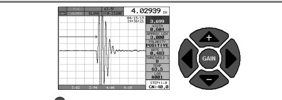
1) Press the Gain key multiple times to increment the Step Size. Note: the Step Size options will advance from low to high which each key press and wrap back around to the beginning option.
