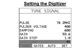
1) Press the MENU key once to activate the menu items tab. Press the MENU key multiple times to tab right and the ESC key multiple times to tab left until the TUNE menu is highlighted and displaying the submenu items.
