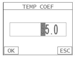
15) Press the **ENTER** key to display the **Digits Edit Box** and adjust the **TEMP COEF**.
