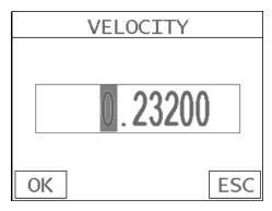
12) Press the **ENTER** key to display the **Digits Edit Box** and adjust the **VELOCITY** of the cal bar.
