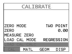
3) Press the **ENTER** key to run the calculation and display the confirmation screen.
