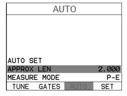
6) Press the **MENU** key multiple times to tab right and the **ESC** key multiple times to tab left until the **AUTO** menu is highlighted and displaying the sub
