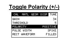
**Note:** Before toggling the **Polarity**, the *MAX II* should be set to the **RF** display view option. The **RF** view will give the user the best opportunity to correctly view the positive and negative cycles of the waveform. Please refer section 12.2 for information on selecting the **Display Views**.
