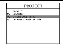
4) Use the **UP** and **DOWN** arrow keys multiple times using the left button wheel to scroll through the project list until the desired **PROJECT** is highlighted.
