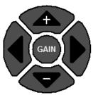
1) Press the **UP** and **DOWN** arrow keys using the right button wheel to increase/decrease the gain value at any time.
